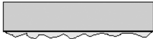
Fig 21. Low Speed Dross Formation
